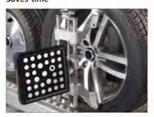
Once the four targets are fitted on the wheels, the complete alignment readings are available within seconds. This allows to carry out more alignments a day – and your investment pays off within short.
